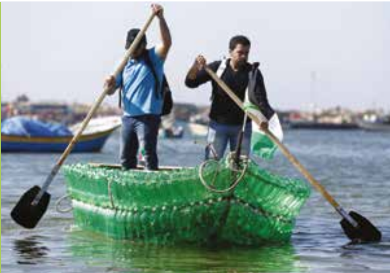
In Gaza, cousins paddle a boat entirely constructed of scrap metal and recycled plastic bottles. The 13-foot vessel, which took three months to build, was improvised by five friends confined by the Israeli siege of the territory.
